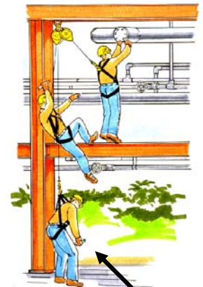
Retractable lifelines can reduce clearance requirements
